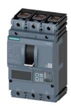
circuit breaker 3VA2 IEC frame 160 breaking capacity class C Icu=110kA @ 415V 3-pole, line protection ETU860, LSIG, In=25A overload protection Ir=10A...25A short-circuit protection Isd=0.6..10x In, Ii=1.5..12x In N conductor protection optionally with external current transformer, up to 160% gr.-fault prot., can be sw. off Ig=0.2...1 x In, tg=0.05-0.8s clamp connection
