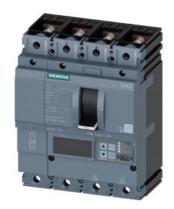
circuit breaker 3VA2 IEC frame 160 breaking capacity class C Icu=110kA @ 415V 4-pole, line protection ETU850, LSI, In=25A overload protection Ir=10A...25A short-circuit protection Isd=0.6..10x In, Ii=1.5..12x In N conductor protection adjustable (OFF, up to 160%) nut keeper kit
