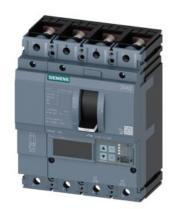
circuit breaker 3VA2 IEC frame 160 breaking capacity class C Icu=110kA @ 415V 4-pole, line protection ETU560, LSIG, In=25A overload protection Ir=10A...25A short-circuit protection Isd=0.6..10x In, Ii=1.5..12x In N conductor protection adjustable (OFF, up to 160%) gr.-fault prot., can be sw. off Ig=0.2...1 x In= tg=0.05-0.8s nut keeper kit
