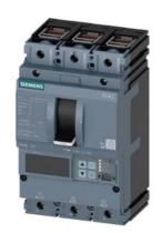
circuit breaker 3VA2 IEC frame 160 breaking capacity class C Icu=110kA @ 415V 3-pole, line protection ETU560, LSIG, In=25A overload protection Ir=10A...25A short-circuit protection Isd=0.6..10x In, Ii=1.5..12x In N conductor protection optionally with external current transformer, up to 160% gr.-fault prot., can be sw. off Ig=0.2...1 x In, tg=0.05-0.8s clamp connection
