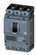
circuit breaker 3VA2 IEC frame 160 breaking capacity class C Icu=110kA @ 415V 3-pole, line protection ETU560, LSIG, In=25A overload protection Ir=10A...25A short-circuit protection Isd=0.6..10x In, Ii=1.5..12x In N conductor protection optionally with external current transformer, up to 160% gr.-fault prot., can be sw. off Ig=0.2...1 x In, tg=0.05-0.8s nut keeper kit
