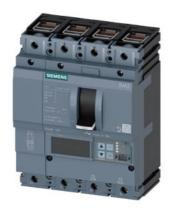
circuit breaker 3VA2 IEC frame 160 breaking capacity class C Icu=110kA @ 415V 4-pole, line protection ETU550, LSI, In=25A overload protection Ir=10A...25A short-circuit protection Isd=0.6..10x In, Ii=1.5..12x In N conductor protection adjustable (OFF, up to 160%) clamp connection
