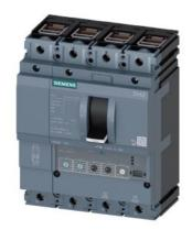
circuit breaker 3VA2 IEC frame 160 breaking capacity class C Icu=110kA @ 415V 4-pole, line protection ETU350, LSI, In=25A overload protection Ir=10A...25A short-circuit protection Isd=1.5...10 x Ir, Ii=12 x In N conductor protection adjustable (OFF, 100%) clamp connection
