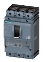
circuit breaker 3VA2 IEC frame 160 breaking capacity class C Icu=110kA @ 415V 3-pole, line protection ETU350, LSI, In=25A overload protection Ir=10A...25A short-circuit protection Isd=1.5...10 x Ir, Ii=12 x In clamp connection
