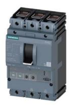
circuit breaker 3VA2 IEC frame 160 breaking capacity class C Icu=110kA @ 415V 3-pole, line protection ETU330, LIG, In=25A overload protection Ir=10A...25A short-circuit protection Ii=1.5...12 x In ground-fault protection Ig=0.6... 1 x In, tg=0.1/0.3s clamp connection
