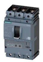
circuit breaker 3VA2 IEC frame 160 breaking capacity class C Icu=110kA @ 415V 3-pole, line protection ETU330, LIG, In=25A overload protection Ir=10A...25A short-circuit protection Ii=1.5...12 x In ground-fault protection Ig=0.6... 1 x In, tg=0.1/0.3s nut keeper kit
