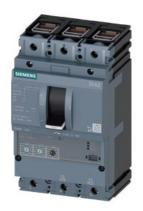
circuit breaker 3VA2 IEC frame 160 breaking capacity class C Icu=110kA @ 415V 3-pole, line protection ETU320, LI, In=25A overload protection Ir=10A...25A short-circuit protection Ii=1.5...12 x In clamp connection
