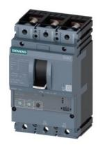
circuit breaker 3VA2 IEC frame 160 breaking capacity class C lcu=110kA @ 415V 3-pole, line protection ETU320, LI, In=25A overload protection Ir=10A...25A short-circuit protection Ii=1.5...12 x In nut keeper kit
