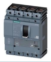
circuit breaker 3VA2 IEC frame 160 breaking capacity class C Icu=110kA @ 415V 4-pole, line protection ETU340, ELISA LI, In=25A overload protection Ir=10A...25A short-circuit protection Ii=15 x In N conductor protection adjustable (OFF, 100%) clamp connection
