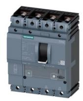
circuit breaker 3VA2 IEC frame 160 breaking capacity class C Icu=110kA @ 415V 4-pole, line protection ETU340, ELISA LI, In=25A overload protection Ir=10A...25A short-circuit protection Ii=15 x In N conductor protection adjustable (OFF, 100%) nut keeper kit
