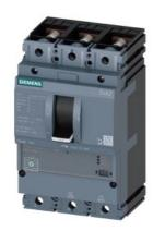
circuit breaker 3VA2 IEC frame 160 breaking capacity class C Icu=110kA @ 415V 3-pole, line protection ETU340, ELISA LI, In=25A overload protection Ir=10A...25A short-circuit protection Ii=15 x In nut keeper kit
