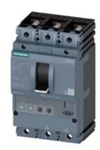
circuit breaker 3VA2 IEC frame 160 breaking capacity class H Icu=85kA @ 415V 3-pole, line protection ETU330, LIG, In=25A overload protection Ir=10A...25A short-circuit protection Ii=1.5...12 x In ground-fault protection Ig=0.6... 1 x In, tg=0.1/0.3s nut keeper kit
