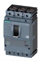
circuit breaker 3VA2 IEC frame 160 breaking capacity class H Icu=85kA @ 415V 3-pole, line protection ETU340, ELISA LI, In=25A overload protection Ir=10A...25A short-circuit protection Ii=15 x In clamp connection
