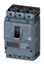
CIRCUIT BREAKER 3VA2 IEC FRAME 160 BREAKING CAPACITY CLASS C ICU=110KA @ 415 V 3-POLE, MOTOR PROTECTION ETU550M, LSI, In=100A OVERLOAD PROTECTION IR=40A ...100A SHORT CIRCUIT PROTECTION ISD=1,2... 15X IN,II=3...15X IN CABLE CONNECTION
