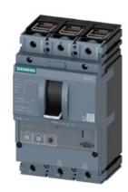
circuit breaker 3VA2 IEC frame 160 breaking capacity class C Icu=110kA @ 415V 3-pole, motor protection ETU350M, LSI, In=100A overload protection Ir=40A...100A short-circuit protection Isd=3...15 x Ir, Ii=15 x In clamp connection
