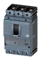
circuit breaker 3VA2 IEC frame 160 breaking capacity class C Icu=110kA @ 415V 3-pole, motor protection ETU350M, LSI, In=100A overload protection Ir=40A...100A short-circuit protection Isd=3...15 x Ir, Ii=15 x In nut keeper kit
