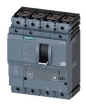
circuit breaker 3VA2 IEC frame 160 breaking capacity class C Icu=110kA @ 415V 4-pole, line protection ETU340, ELISA LI, In=100A overload protection Ir=40A...100A short-circuit protection Ii=15 x In N conductor protection adjustable (OFF, 50%, 100%) clamp connection
