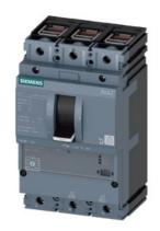
circuit breaker 3VA2 IEC frame 160 breaking capacity class C Icu=110kA @ 415V 3-pole, line protection ETU340, ELISA LI, In=100A overload protection Ir=40A...100A short-circuit protection Ii=15 x In clamp connection
