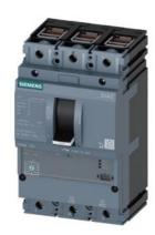
circuit breaker 3VA2 IEC frame 160 breaking capacity class H Icu=85kA @ 415V 3-pole, line protection ETU340, ELISA LI, In=100A overload protection Ir=40A...100A short-circuit protection Ii=15 x In clamp connection
