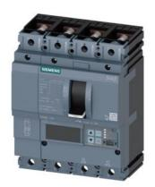
circuit breaker 3VA2 IEC frame 100 breaking capacity class L Icu=150kA @ 415V 4-pole, line protection ETU860, LSIG, In=63A overload protection Ir=25A...63A short-circuit protection Isd=0.6...10x In, Ii=1.5...12x In N conductor protection adjustable (OFF, up to 160%) gr.-fault prot., can be sw. off Ig=0.25...1 x In= tg=0.05-0.8s nut keeper kit
