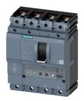
circuit breaker 3VA2 IEC frame 100 breaking capacity class L lcu=150kA @ 415V 4-pole, line protection ETU350, LSI, ln=63A overload protection lr=25A...63A short-circuit protection lsd=1.5...10 x lr, li=12 x ln N conductor protection adjustable (OFF, 100%) nut keeper kit
