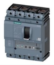
circuit breaker 3VA2 IEC frame 100 breaking capacity class L Icu=150kA @ 415V 4-pole, line protection ETU330, LIG, In=63A overload protection Ir=25A...63A short-circuit protection Ii=1.5...12 x In N conductor protection adjustable (OFF, 100%) ground-fault protection Ig=0.25...1 x In= tg=0.1/0.3s clamp connection
