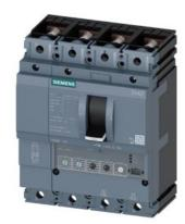
circuit breaker 3VA2 IEC frame 100 breaking capacity class L Icu=150kA @ 415V 4-pole, line protection ETU330, LIG, In=63A overload protection Ir=25A...63A short-circuit protection Ii=1.5...12 x In N conductor protection adjustable (OFF, 100%) ground-fault protection Ig=0.25...1 x In= tg=0.1/0.3s nut keeper kit
