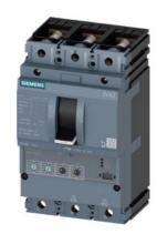
circuit breaker 3VA2 IEC frame 100 breaking capacity class L Icu=150kA @ 415V 3-pole, line protection ETU330, LIG, In=63A overload protection Ir=25A...63A short-circuit protection Ii=1.5...12 x In ground-fault protection Ig=0.25... 1 x In, tg=0.1/0.3s nut keeper kit
