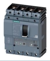
circuit breaker 3VA2 IEC frame 100 breaking capacity class L Icu=150kA @ 415V 4-pole, line protection ETU320, LI, In=63A overload protection Ir=25A...63A short-circuit protection Ii=1.5...12 x In N conductor protection adjustable (OFF, 100%) nut keeper kit
