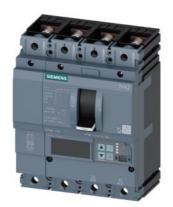
circuit breaker 3VA2 IEC frame 100 breaking capacity class L Icu=150kA @ 415V 4-pole, line protection ETU860, LSIG, In=25A overload protection Ir=10A...25A short-circuit protection Isd=0.6..10x In, Ii=1.5..12x In N conductor protection adjustable (OFF, up to 160%) gr.-fault prot., can be sw. off Ig=0.2...1 x In= tg=0.05-0.8s nut keeper kit
