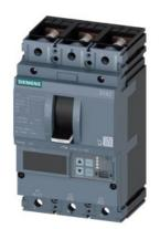
circuit breaker 3VA2 IEC frame 100 breaking capacity class L Icu=150kA @ 415V 3-pole, line protection ETU860, LSIG, In=25A overload protection Ir=10A...25A short-circuit protection Isd=0.6..10x In, Ii=1.5..12x In N conductor protection optionally with external current transformer, up to 160% gr.-fault prot., can be sw. off Ig=0.2...1 x In, tg=0.05-0.8s nut keeper kit
