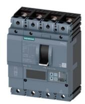
circuit breaker 3VA2 IEC frame 100 breaking capacity class L Icu=150kA @ 415V 4-pole, line protection ETU850, LSI, In=25A overload protection Ir=10A...25A shortcircuit protection Isd=0.6..10x In, Ii=1.5..12x In N conductor protection adjustable (OFF, up to 160%) nut keeper kit
