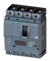
circuit breaker 3VA2 IEC frame 100 breaking capacity class L Icu=150kA @ 415V 4-pole, line protection ETU550, LSI, In=25A overload protection Ir=10A...25A short-circuit protection Isd=0.6..10x In, Ii=1.5..12x In N conductor protection adjustable (OFF, up to 160%) nut keeper kit
