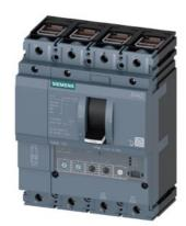
circuit breaker 3VA2 IEC frame 100 breaking capacity class L Icu=150kA @ 415V 4-pole, line protection ETU350, LSI, In=25A overload protection Ir=10A...25A short-circuit protection Isd=1.5...10 x Ir, Ii=12 x In N conductor protection adjustable (OFF, 100%) clamp connection
