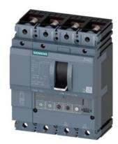
circuit breaker 3VA2 IEC frame 100 breaking capacity class L Icu=150kA @ 415V 4-pole, line protection ETU350, LSI, In=25A overload protection Ir=10A...25A shortcircuit protection Isd=1.5...10 x Ir, Ii=12 x In N conductor protection adjustable (OFF, 100%) nut keeper kit
