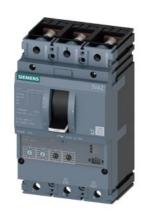
circuit breaker 3VA2 IEC frame 100 breaking capacity class L Icu=150kA @ 415V 3-pole, line protection ETU350, LSI, In=25A overload protection Ir=10A...25A short-circuit protection Isd=1.5...10 x Ir, Ii=12 x In nut keeper kit
