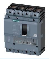
circuit breaker 3VA2 IEC frame 100 breaking capacity class L Icu=150kA @ 415V 4-pole, line protection ETU330, LIG, In=25A overload protection Ir=10A...25A short-circuit protection Ii=1.5...12 x In N conductor protection adjustable (OFF, 100%) ground-fault protection Ig=0.6...1 x In= tg=0.1/0.3s clamp connection
