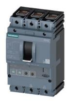
circuit breaker 3VA2 IEC frame 100 breaking capacity class L Icu=150kA @ 415V 3-pole, line protection ETU330, LIG, In=25A overload protection Ir=10A...25A short-circuit protection Ii=1.5...12 x In ground-fault protection Ig=0.6... 1 x In, tg=0.1/0.3s clamp connection
