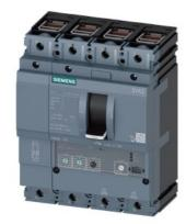
circuit breaker 3VA2 IEC frame 100 breaking capacity class L Icu=150kA @ 415V 4-pole, line protection ETU320, LI, In=25A overload protection Ir=10A...25A short-circuit protection Ii=1.5...12 x In N conductor protection adjustable (OFF, 100%) clamp connection
