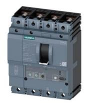
circuit breaker 3VA2 IEC frame 100 breaking capacity class L Icu=150kA @ 415V 4-pole, line protection ETU320, LI, In=25A overload protection Ir=10A...25A short-circuit protection Ii=1.5...12 x In N conductor protection adjustable (OFF, 100%) nut keeper kit
