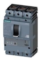
circuit breaker 3VA2 IEC frame 100 breaking capacity class L Icu=150kA @ 415V 3-pole, line protection ETU320, LI, In=25A overload protection Ir=10A...25A short-circuit protection Ii=1.5...12 x In clamp connection
