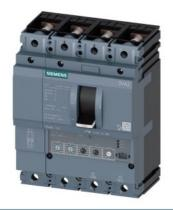
circuit breaker 3VA2 IEC frame 100 breaking capacity class L Icu=150kA @ 415V 4-pole, line protection ETU330, LIG, In=100A overload protection Ir=40A...100A short-circuit protection Ii=1.5...12 x In N conductor protection adjustable (OFF, 50%, 100%) ground-fault protection Ig=0.2...1 x In= tg=0.1/0.3s nut keeper kit
