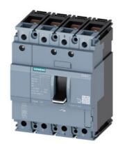
circuit breaker 3VA1 IEC frame 160 breaking capacity class M Icu=55kA @ 415V 4-pole, line protection TM210, FTFM, In=16A overload protection Ir=16A fixed short-circuit protection Ii=20 x In N conductor protection 100% nut keeper kit
