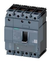
circuit breaker 3VA1 IEC frame 160 breaking capacity class M Icu=55kA @ 415V 4-pole, line protection TM220, ATFM, In=16A overload protection Ir=11A...16A short-circuit protection Ii=20 x In N conductor unprotected nut keeper kit
