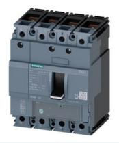
circuit breaker 3VA1 IEC frame 160 breaking capacity class S Icu=36kA @ 415V 4-pole, line protection TM220, ATFM, In=16A overload protection Ir=11A...16A short-circuit protection Ii=20 x In N conductor unprotected nut keeper kit
