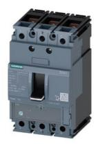
circuit breaker 3VA1 IEC frame 160 breaking capacity class N Icu=25kA @ 415V 3-pole, line protection TM220, ATFM, In=16A overload protection Ir=11A...16A short-circuit protection Ii=20 x In nut keeper kit
