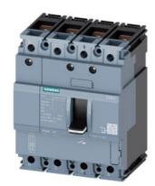
circuit breaker 3VA1 IEC frame 160 breaking capacity class S Icu=36kA @ 415V 4-pole, line protection TM210, FTFM, In=80A overload protection Ir=80A fixed short-circuit protection Ii=10 x In N conductor protection 100% nut keeper kit
