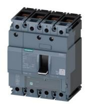
circuit breaker 3VA1 IEC frame 160 breaking capacity class S Icu=36kA @ 415V 4-pole, line protection TM220, ATFM, In=80A overload protection Ir=56A...80A short-circuit protection Ii=10 x In N conductor unprotected nut keeper kit
