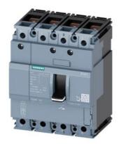
circuit breaker 3VA1 IEC frame 160 breaking capacity class M Icu=55kA @ 415V 4-pole, line protection TM210, FTFM, In=63A overload protection Ir=63A fixed short-circuit protection Ii=10 x In N conductor protection 100% nut keeper kit
