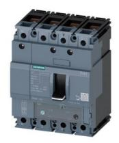
circuit breaker 3VA1 IEC frame 160 breaking capacity class S Icu=36kA @ 415V 4-pole, line protection TM240, ATAM, In=63A overload protection Ir=44A...63A short-circuit protection Ii=5...10 x In N conductor protection 100% nut keeper kit
